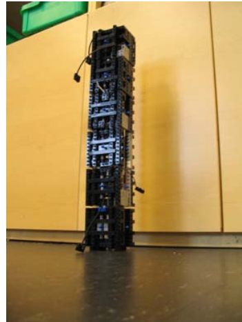
Fig. 6. This figure shows six modules connected to form a module bone that can be used to give the modular robot structural strength. Note that this is possible because of the large contact surface and fairly strong connections between neighbouring modules.
